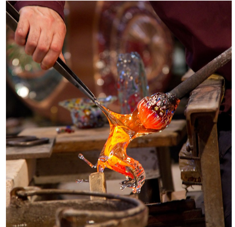
Typical glass horse being shaped
